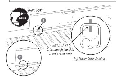
Remove temporary Rail from both Rack Plates. Drill remaining hole in both Plates and install Hardware (G).
