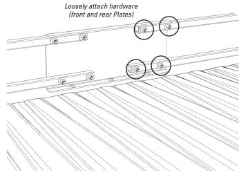
FULLY TIGHTEN AFTER ALL 16 BOLTS ARE INSTALLED.
