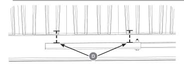
Double check alignment by measuring from Plate to Top Edge
